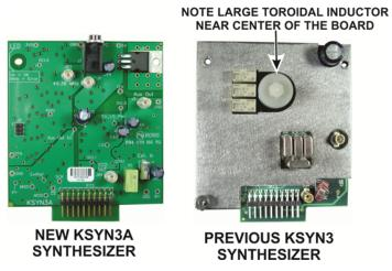
Page 52: Delete the first step and figure 72. The stiffener is not used on the new KSYN3A board.
